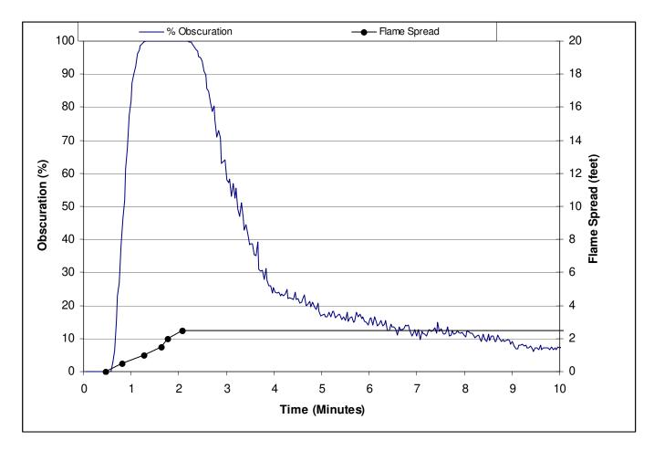
Test No. 1 09CA48646 / SV18041 10260922 Flame Spread Index: 10 Smoke Developed Index: 400 Max. Flame Spread: 2.5
