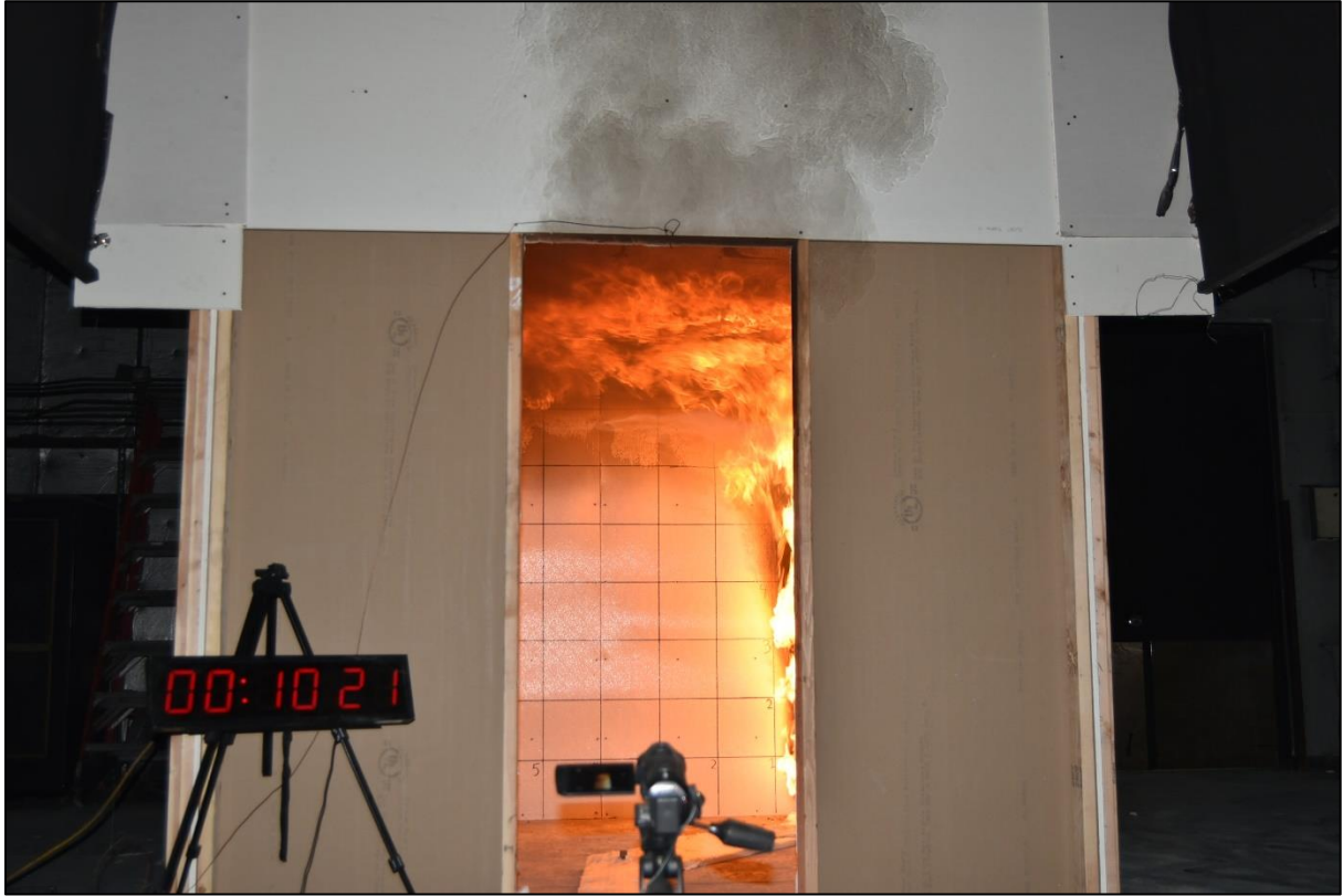
Figure A-7. Test at 10 min 21 s, Burner Output of 300 kW.
