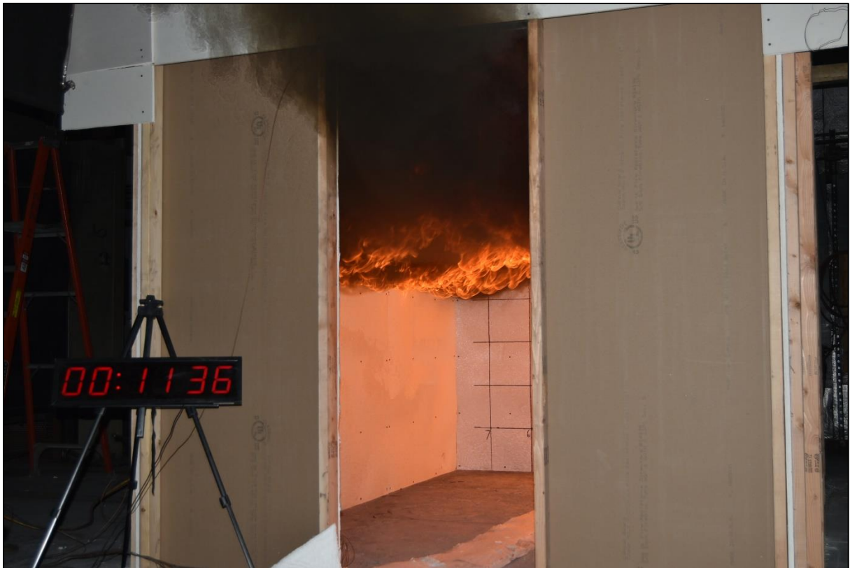
Figure A-8. Test at 11 min 36 s, Burner Output of 300 kW.
