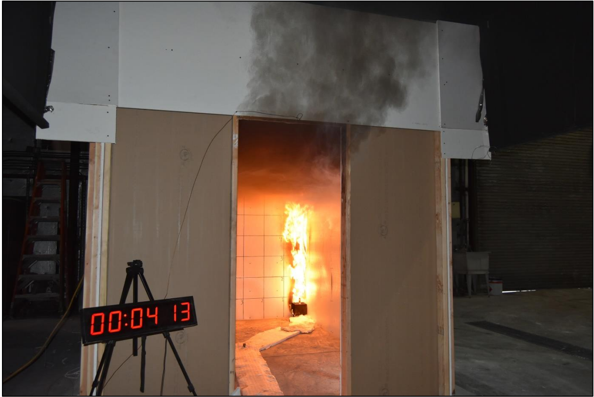
Figure A-5. Test at 4 min 13 s, Burner Output of 100 kW.
