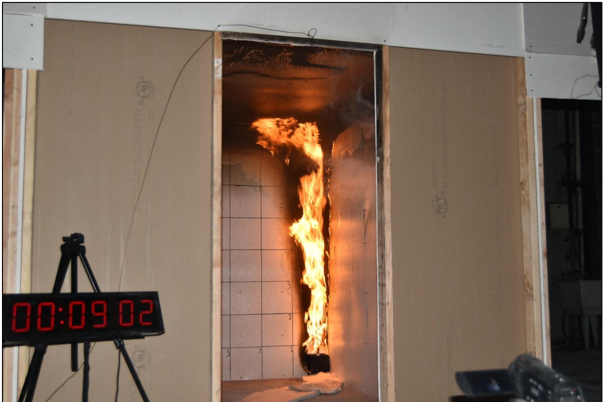
Figure A-6. Test at 9 min 2 s, Burner Output of 100 kW.
