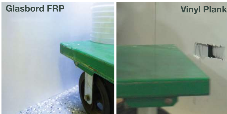
IMPACT RESISTANCE WALL TEST WITH FLATBED CART
