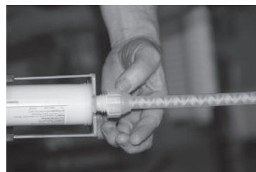
FIGURA 14: ATTACH STATIC MIXING TIP
